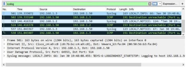
**Note**: The Destination Unreachable messages are host 192.168.1.50, telling the devices that there is not actually a Syslog server running at this IP address.
